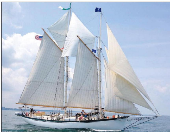
The Appledore IV's rig height is 76 feet. The ship weighs 48 tons and has a hull made of steel.
